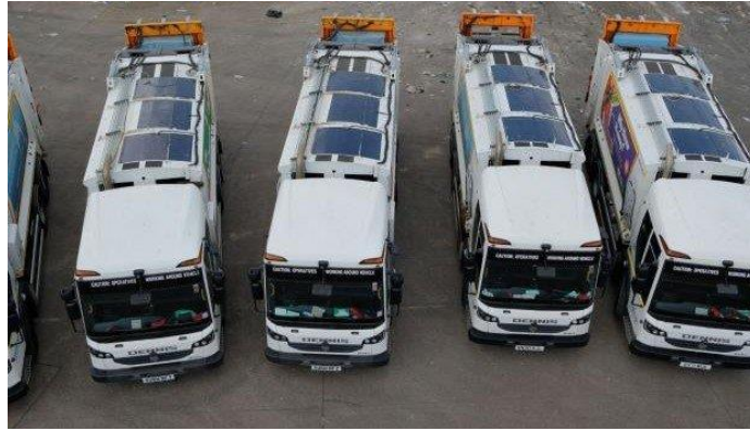
Figure 6. Solar panels installed on Stevenage's refuse collection lorries
